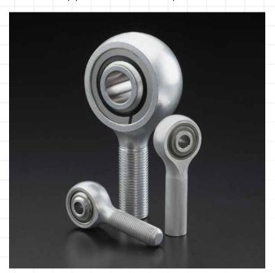
Heim® Ball Bearing Rod Ends are precision ground to tight tolerances for applications requiring selfalignment, low torque and reduced radial clearance. They are greased and equipped with PTFE seals bonded to corrosion resistant caps.
