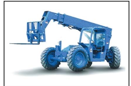
Typical DuraLube Application — Self-lubricated bearings used on hydraulic cylinder rod eyes for tele-handlers.
