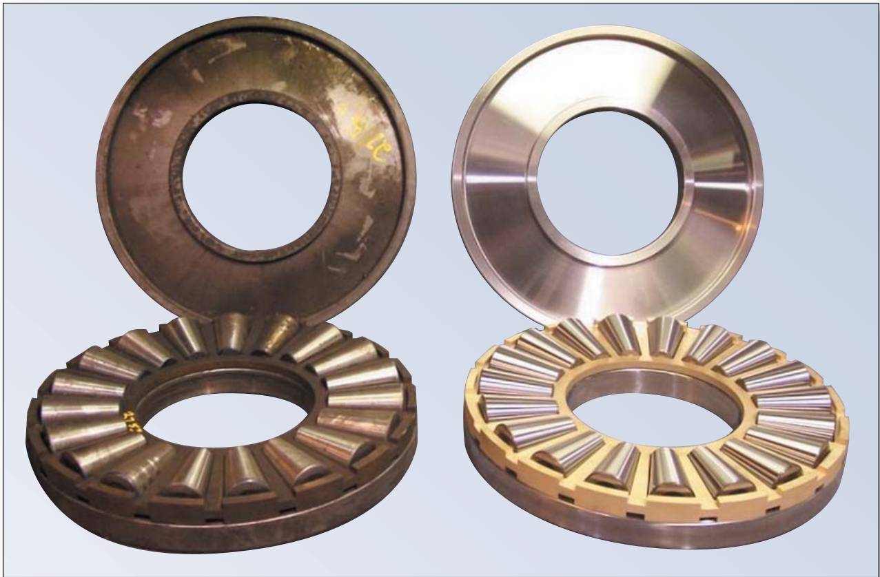
Tapered roller thrust bearing — before and after refurbishment.
