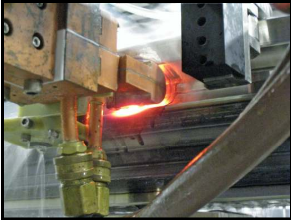
Figure 8 - Induction hardening of a ball path.
