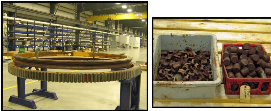
Figure 1 - Bearing races, rollers and separators received for repair.
