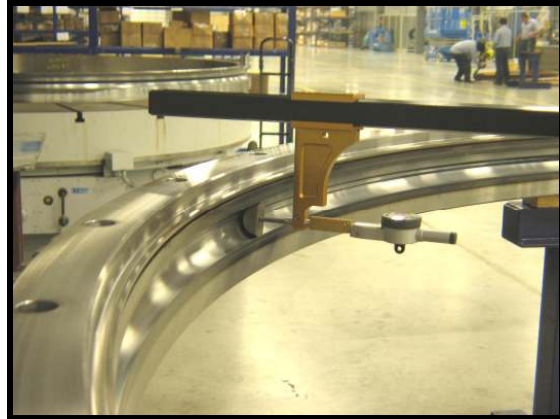
Figure 6 - Measuring ball track diameter.
