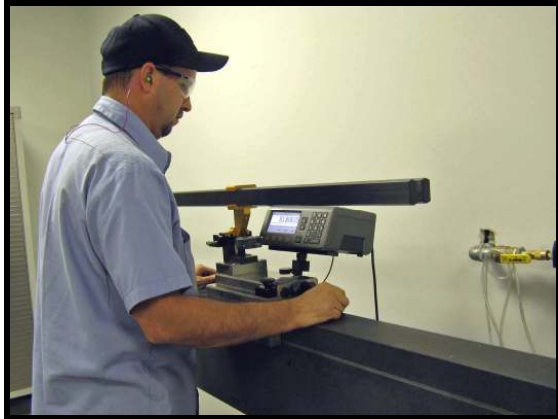
Figure 5 - Setting diameter dimension gauge
