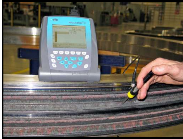
Figure 3 - Measuring the hardness of the raceway.
